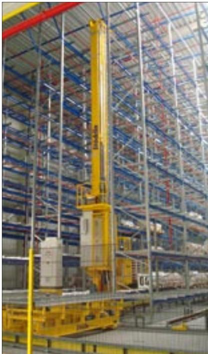
*A new fully automatic stock system for raw material storage in the just-completed second production hall*
