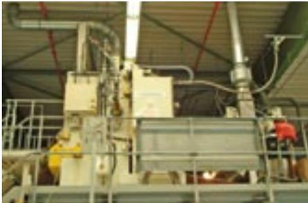
*Electronic beam curing unit*
