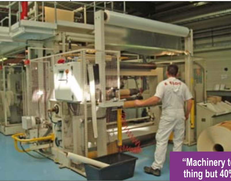
DTS staff inspects the laminate after the electron beam curing process
