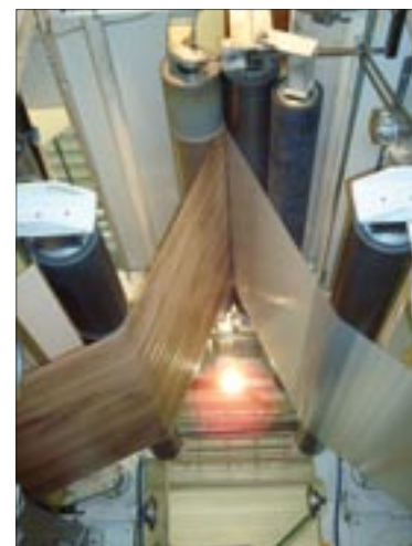
... laminating of impregnated décor paper and release foil together
